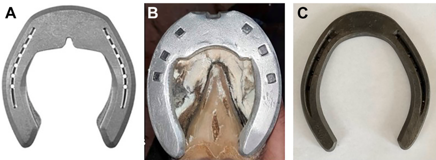
Fig. 2. Examples of (A) manufactured, (B) handmade, and (C) modified keg horseshoe with increased ground surface area in the toe region. (Images courtesy of [A] Grand Circuit Products. [B] Iván D. Gómez.)
